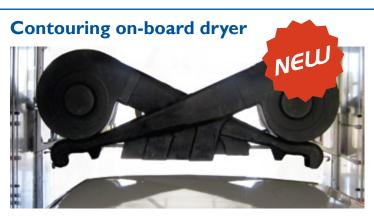
→ Tracks vehicle from the optimal distance to minimize energy consumption while avoiding obstacles such as antennas and roof racks. AquaDri® static on-board and freestanding dryers are also available for the SoftWash XT.
