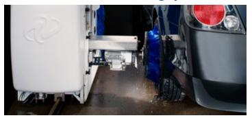
➔ Resolves the number one complaint from consumers: dirty wheels. Wheel brushes with integrated rim spraying rotate both directions to clean convoluted wheel surfaces and allow the operator to charge more for the premium wash package.
